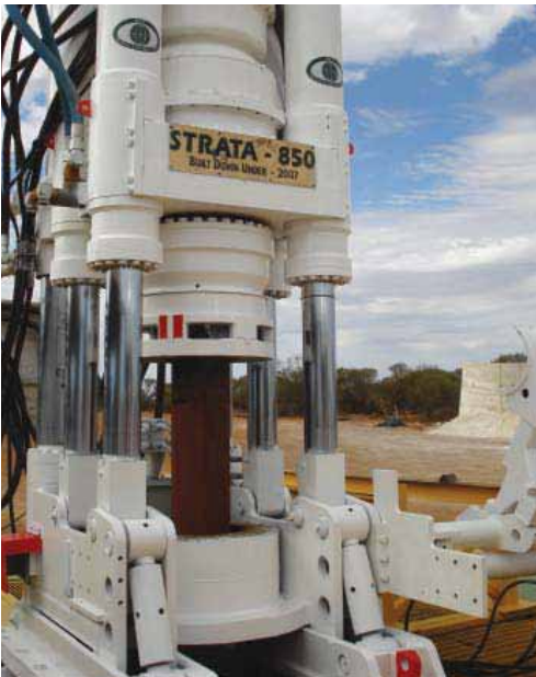
Strata 850 raise borer manufactured by RUC Cementation
